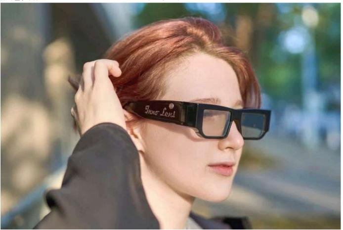
Wearers of the liquid-crystal bifocals can refocus by simply pressing the switch button on the specs' right arm. Credit: Y.-H. Lin *et al./Phys. Rev. Appl.*
